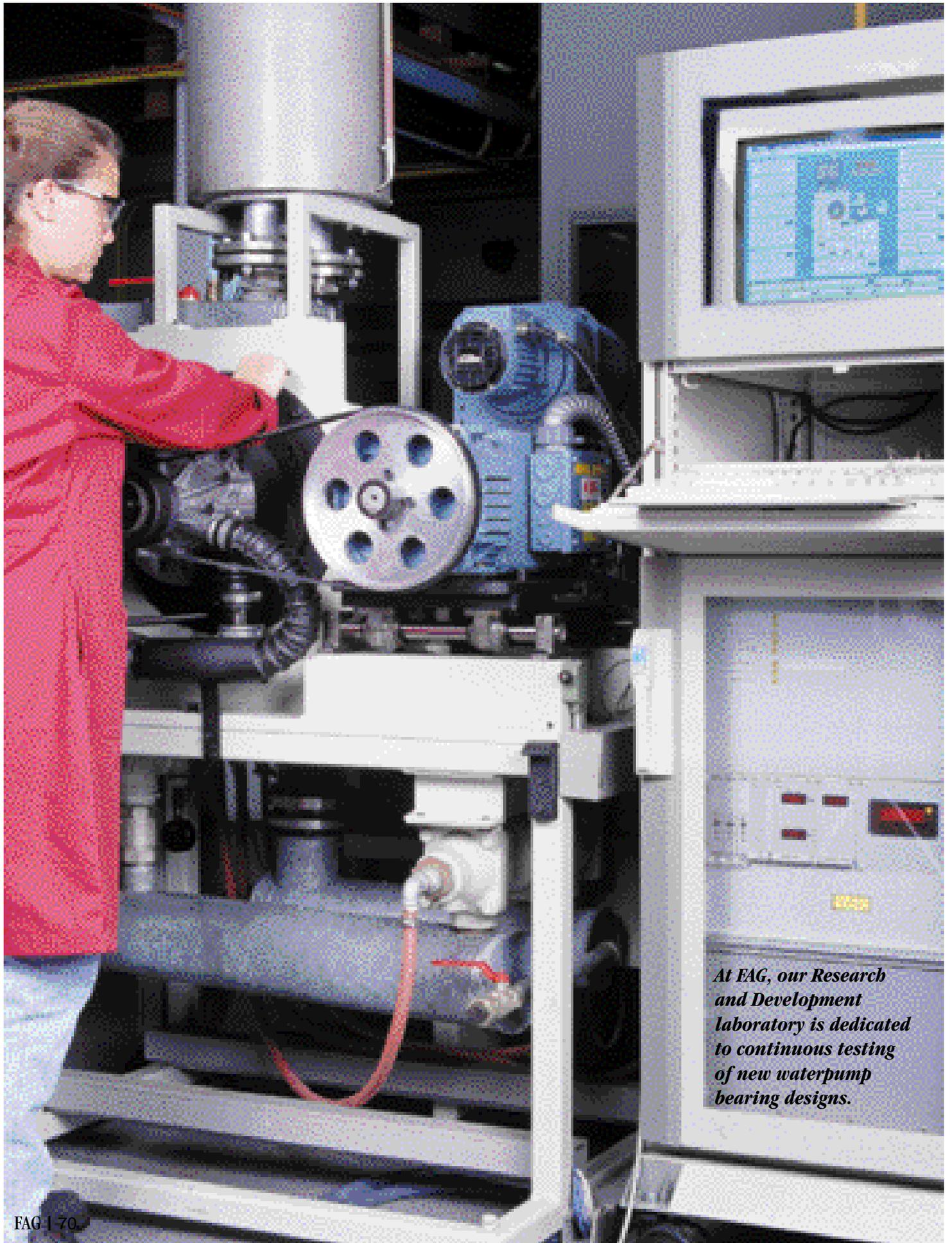
*At FAG, our Research and Development laboratory is dedicated to continuous testing of new waterpump bearing designs.*
