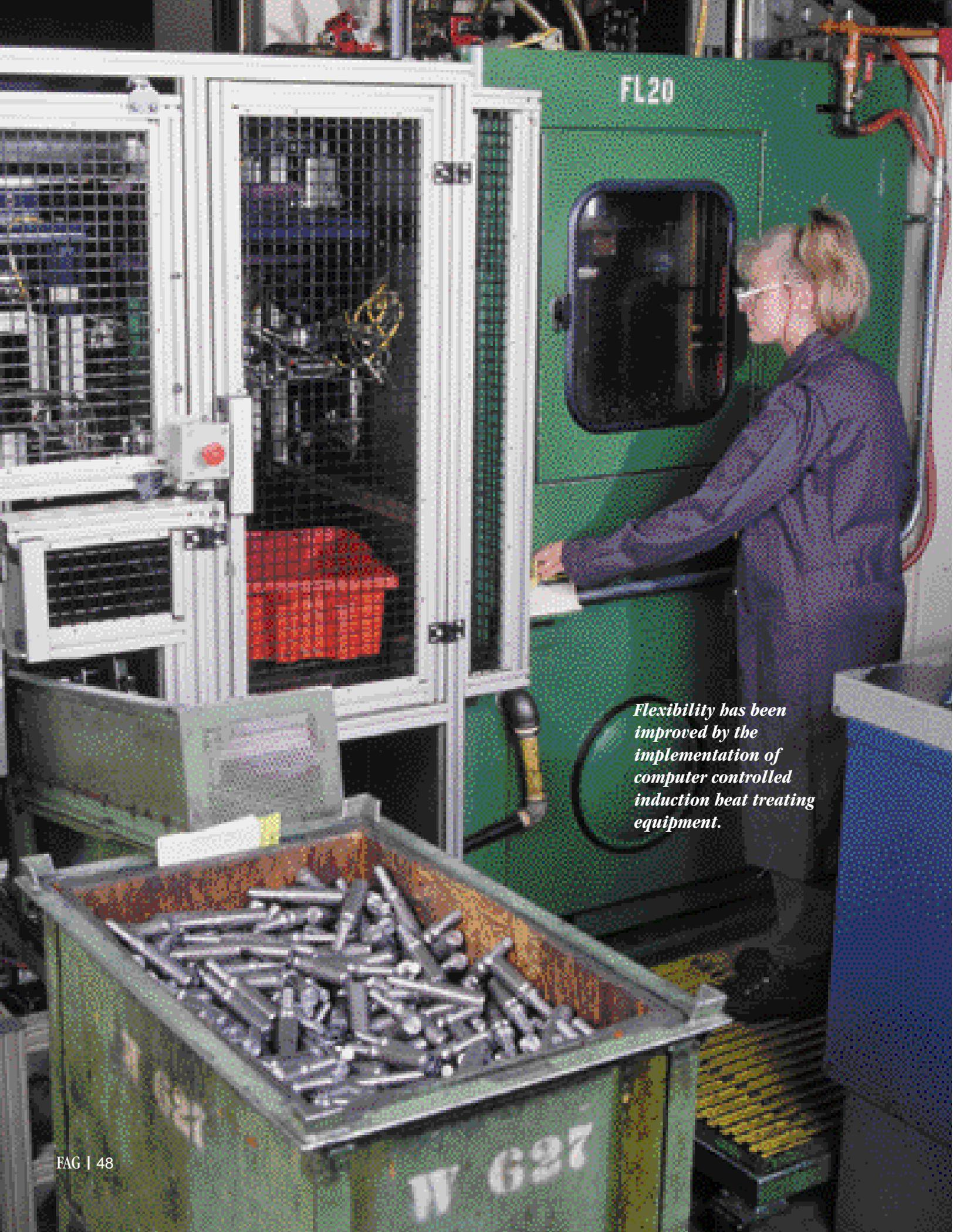
*Flexibility has been improved by the implementation of computer controlled induction heat treating equipment.*
