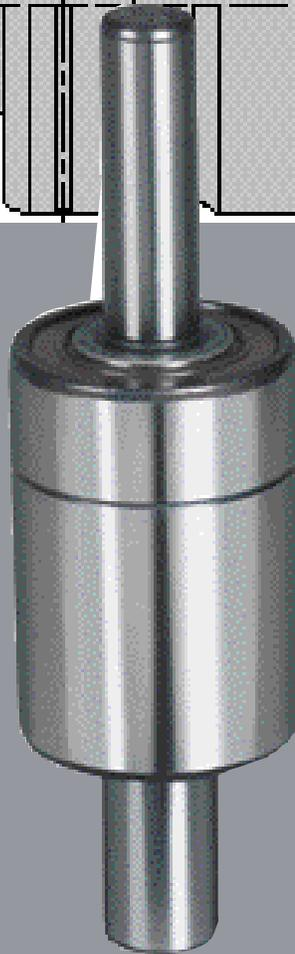
*A WNS bearing consists of a ball / roller internal design. This bearing utilizes a roller complement for increased radial load carrying ability. The “S” represents a special design and is associated with any ball / roller bearing that does not offer standard outer ring or shaft dimensions. Orientation of ball raceway and roller raceway may vary.*
