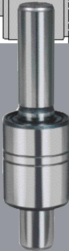
*The W family consists of a ball / ball internal design. Standard design offers a 5/8" main shaft diameter, 1.1811" outer ring diameter, and a 1.530" outer ring length. This bearing is typically used in automotive water pump applications. Some W bearings are available with special features.*
