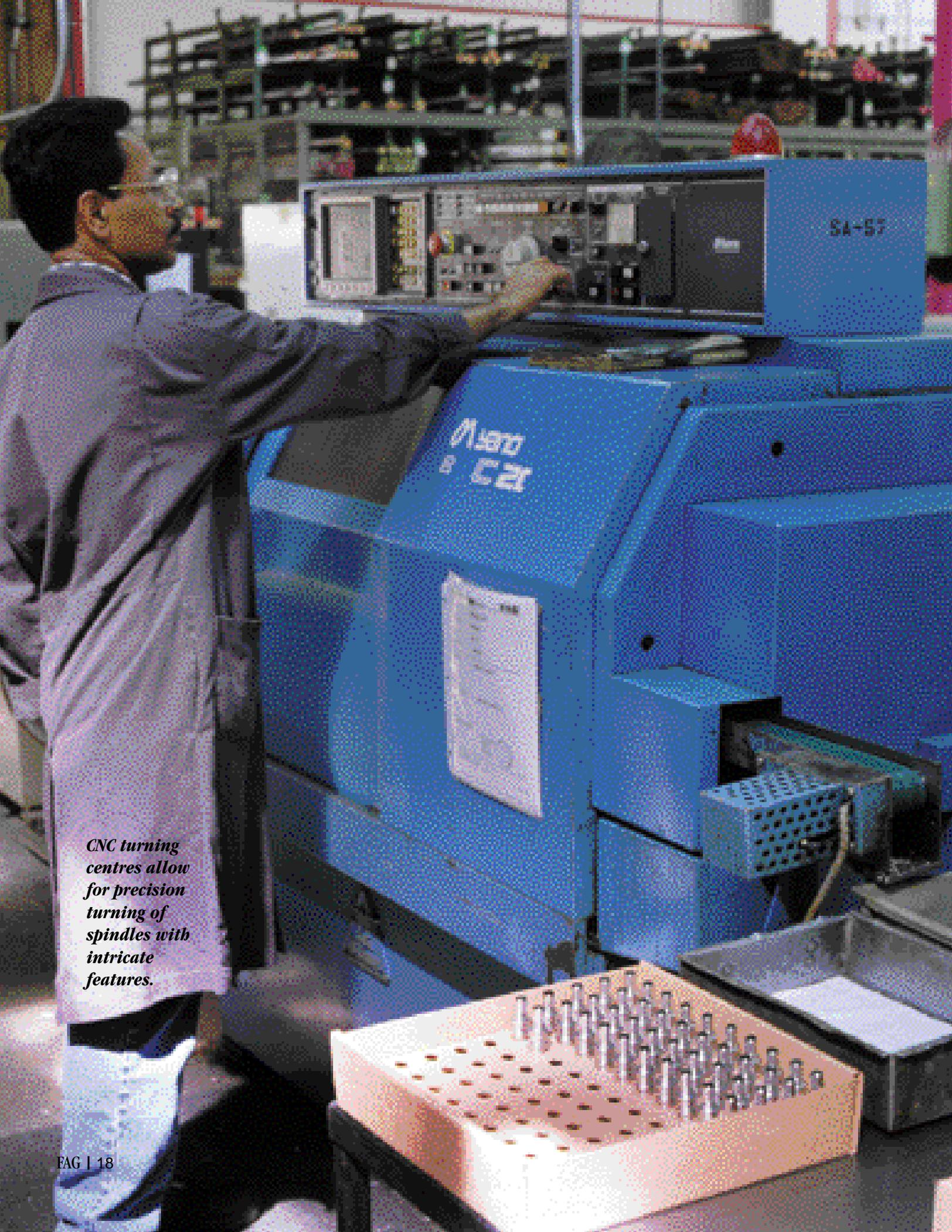
*CNC turning centres allow for precision turning of spindles with intricate features.*
