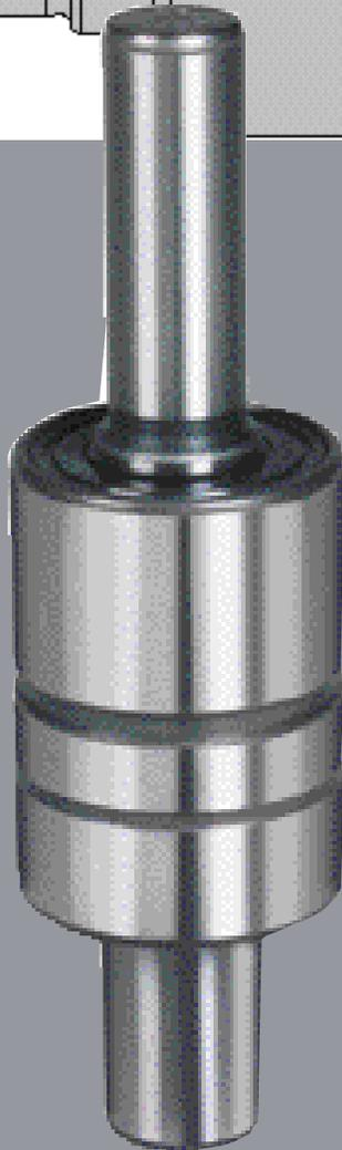
*The WK bearing is essentially a “king size” W bearing that features a ball / ball internal design. Standard dimensions consist of a 1.5000" outer ring diameter and a 2.125" outer ring length. The standard shaft diameter size is 3/4". Larger rolling elements and envelope dimensions allow for higher load carrying ability. This bearing is typically used in automotive water pump applications. Some special designs are available that allow this bearing family to be used in many other applications.*
