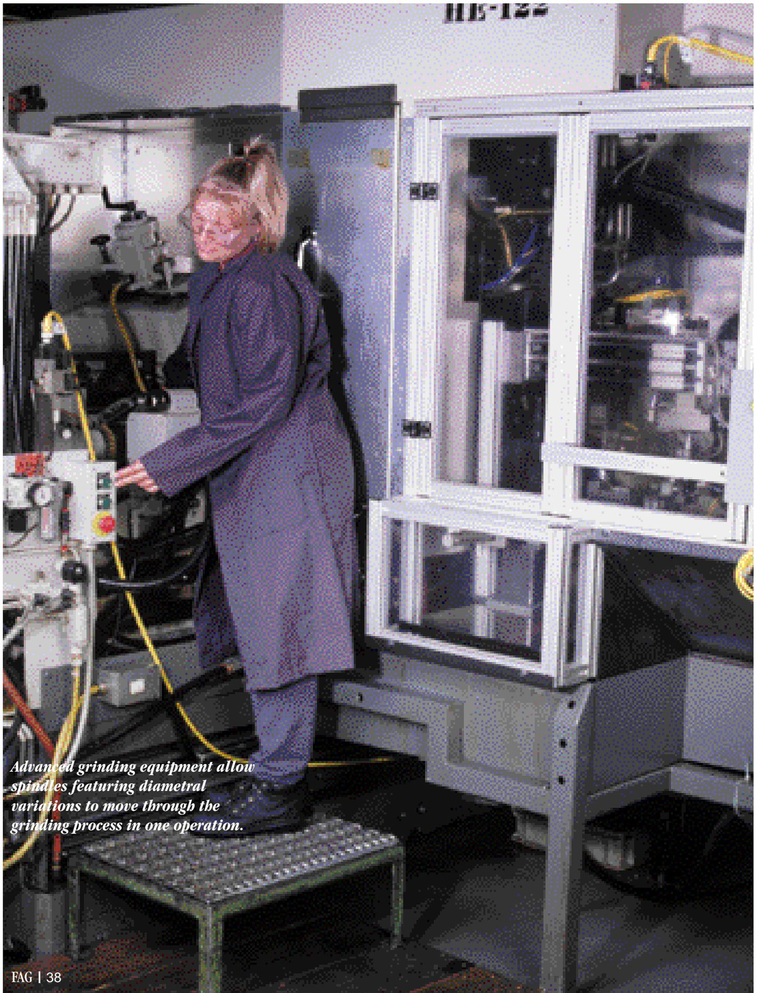
*Advanced grinding equipment allow spindles featuring diametral variations to move through the grinding process in one operation.*
