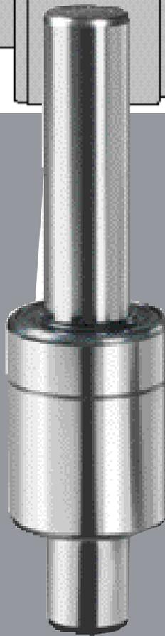
*The WN family consists of a ball / roller internal design. Standard design offers a 5/8" main shaft diameter, 1.1811" outer ring diameter, and a 1.529" outer ring length. This bearing utilizes a ball / roller design for increased radial load carrying ability. Some WN bearings are available with special features.*
