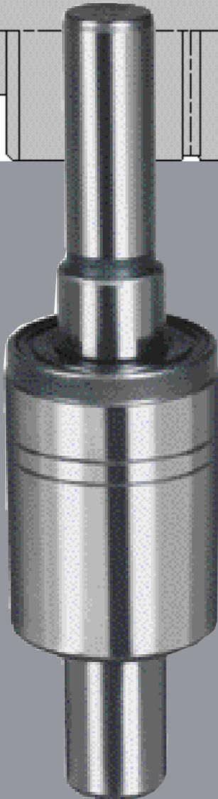
*The WKN bearing is essentially a “king size” WN bearing that features a ball / roller internal design. Standard dimensions consist of a 1.5000" outer ring diameter and a 2.125" outer ring length. Standard shaft diameter size is 3/4". The addition of a roller increases the radial load capacity of the bearing and makes this design extremely versatile for many different applications.*
